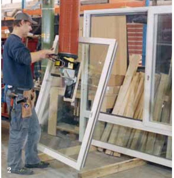
3. Low headroom and more or less no operating space? The VacuMove transformed the task of moving 125 lbs panels to a punching machine into a one-man job.
