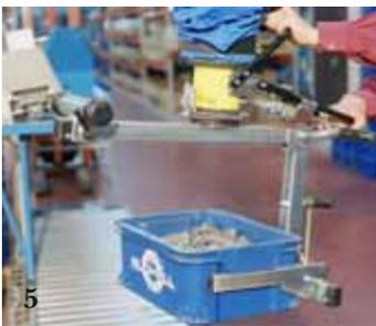
5. A VacuMove with a special tool attached for handling crates. This particular unit is equipped with a fast coupling to allow fast changes between the crate tool and another suction foot for boxes.
