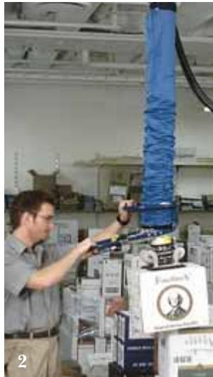
2. Retailers of alcoholic beverages use the VacuMove to handle boxes, crates and kegs. These units are equipped with a specially designed handle and are delivered with lightweight, lowbuilt aluminum jib cranes and bridge crane systems.
