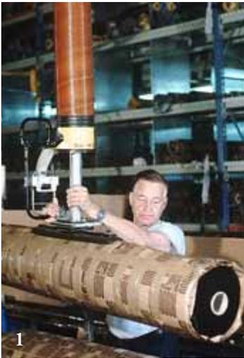
1. A typical installation for objects on which the suction foot must be placed on a curved area. This type of roll-handling is common in industries for the interior decoration i.e carpets, wallpaper. Most often a two-man job before VacuMove is installed.
