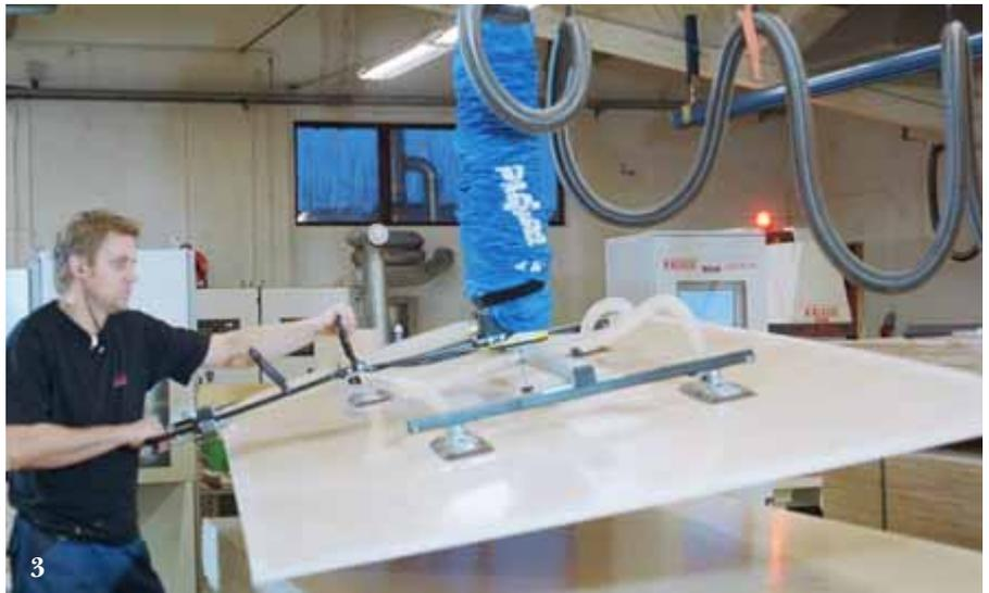
4. The lumber industry depends on VacuMove to lift and move awkwardly large and heavy parts of primary produce. This beautiful piece of wood weighs 550 lbs!
